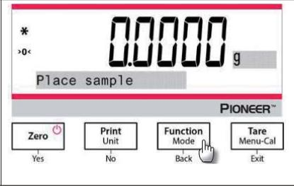
6. Remove the reference sample and place the test object on the pan. The ratio of the test object to the reference sample weight is displayed as a percentage.
