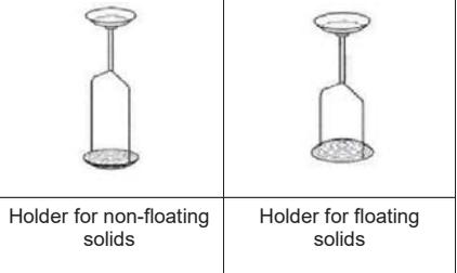
**Note:** Lower the sample down into the liquid until it is fully submerged.
