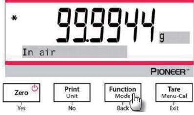
2. Weigh the sample submerged in the liquid using the balance and the density determination kit.
