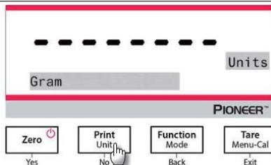
3. Press **Yes** to set the unit displayed to the weighing unit.
