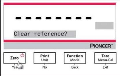
4. Place the reference sample on the pan to display the weight. When the reading is stable, the \* will appear.
