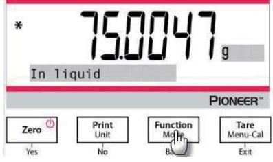
3. Press the **Function / Mode** button to get the density of the sample. After completion of the test, press the **Function / Mode** button to test a new sample.
