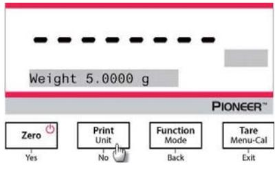
1. Weigh the oiled sample in the air with the balance and the density determination kit.
