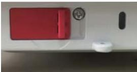
**Note:** This switch is also used in conjunction with the Legal for Trade menu item. When the Legal for Trade menu is set to ON, the switch must be set to the On position to prevent calibration and changes to metrologically significant settings.
